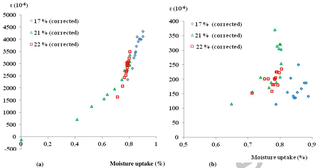
**Figure 7.** Evolutions of the strain as a function of moisture content for the composite specimens instrumented perpendicularly (a) and parallel (b) to the reinforcing fibres.
