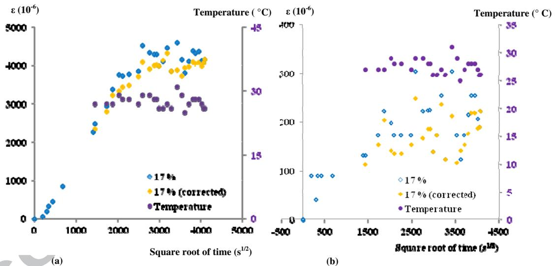
**Figure 6.** Strains evolution as a function of square root of time for the composite specimens instrumented perpendicularly (a) and parallel (b) to the reinforcing fibres.
