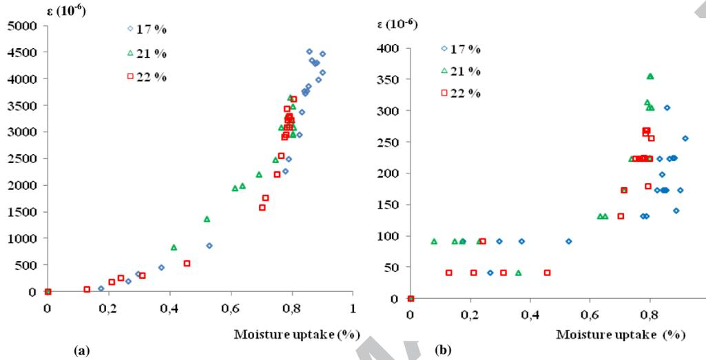
**Figure 4.** Strain as a function of moisture uptake for composite specimens instrumented perpendicularly (a) and parallel (b) to the unidirectional fibres.
