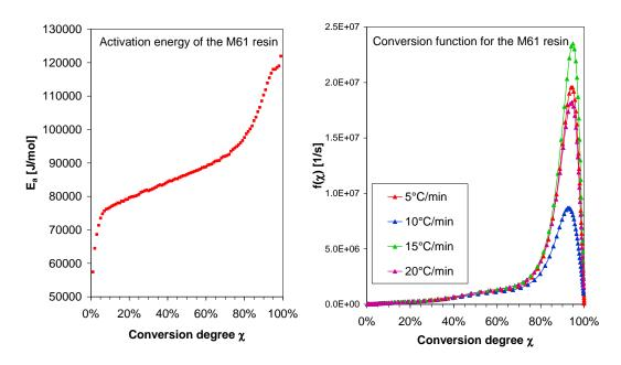
Figure 4: (a) Activation energy (isoconversional method) (b) Conversion functions for the MFK method
