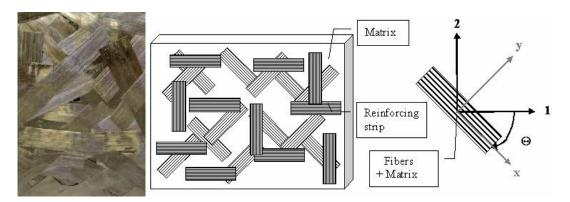
Figure 1: Schematic description of the studied material microstructure
