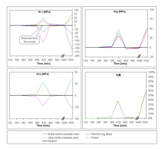
Figure 9: Time dependent evolutions of the local stress states during the curing process, computed for the case #2.
