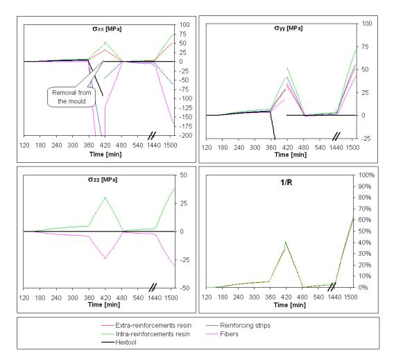
Figure 10: Time dependent evolutions of the local stress states during the curing process, computed for the case #3.
