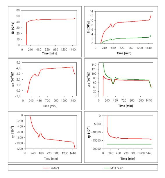
Figure 7: Evolutions of the material effective properties during the cure process
