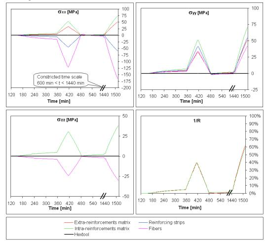
Figure 8: Time dependent evolutions of the local stress states during the curing process, computed for the case #1.
