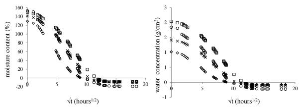
**Fig.8** Desorption curves of natural fibres (♦sisal, ○jute, ×flax, □ hemp)
