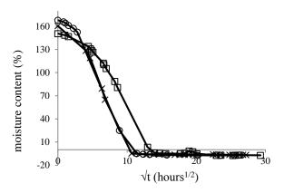
**Fig.10** Cycling results for jute fibre bundles ( $\Box 1^{st}$  cycle,  $\times 2^{nd}$  cycle,  $\bigcirc 3^{rd}$  cycle)
