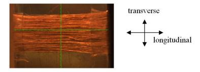
Fig.2 Flax sample used for X-Ray analysis
