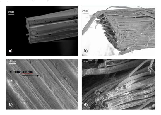
Fig.7 SEM pictures of a) Jute, b) Sisal c) Flax and d) Hemp bundles
