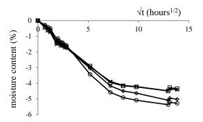
**Fig.9** Determination of initial water in fibres (♦sisal, ○jute, ×flax, □ hemp)
