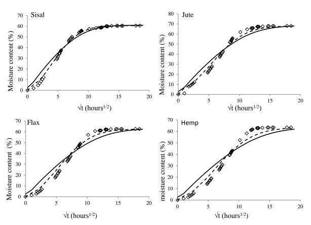
Fig.11 Results for diffusion in immersion (◊ experimental results, --- Langmuir's model, — Fick's model)
