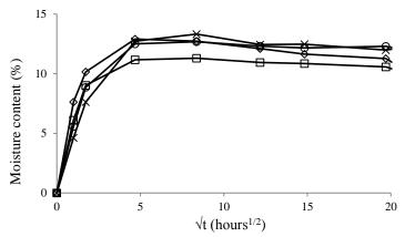
**Fig.12** Absorption kinetics of natural fibres in hygrothermal conditions: RH = 80 %, T = 23°C ( $\diamond$ sisal,  $\circ$ jute,  $\times$ flax,  $\Box$  hemp,)
