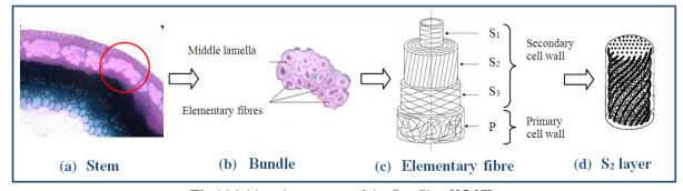
Fig.1 Multi-scale structure of the flax fibre [25,27]
