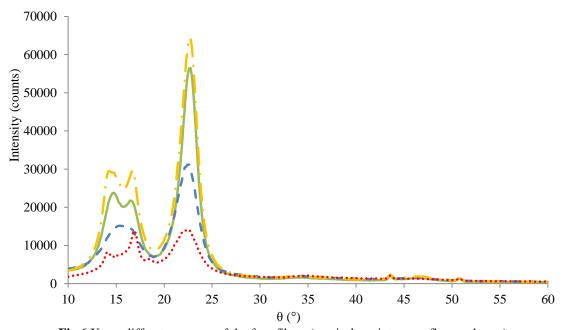
Fig.6 X-ray diffractogramms of the four fibres (··· sisal, --- jute, --· flax, -- hemp)
