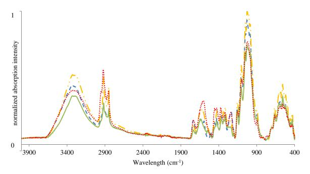
Fig.5 FTIR spectrum of ··· sisal, --- jute, -·· flax, -- hemp fibres
