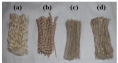
Fig.4 Specimens aged in hygrothermal environments (a) sisal, (b) jute, (c) flax, (d) hemp
